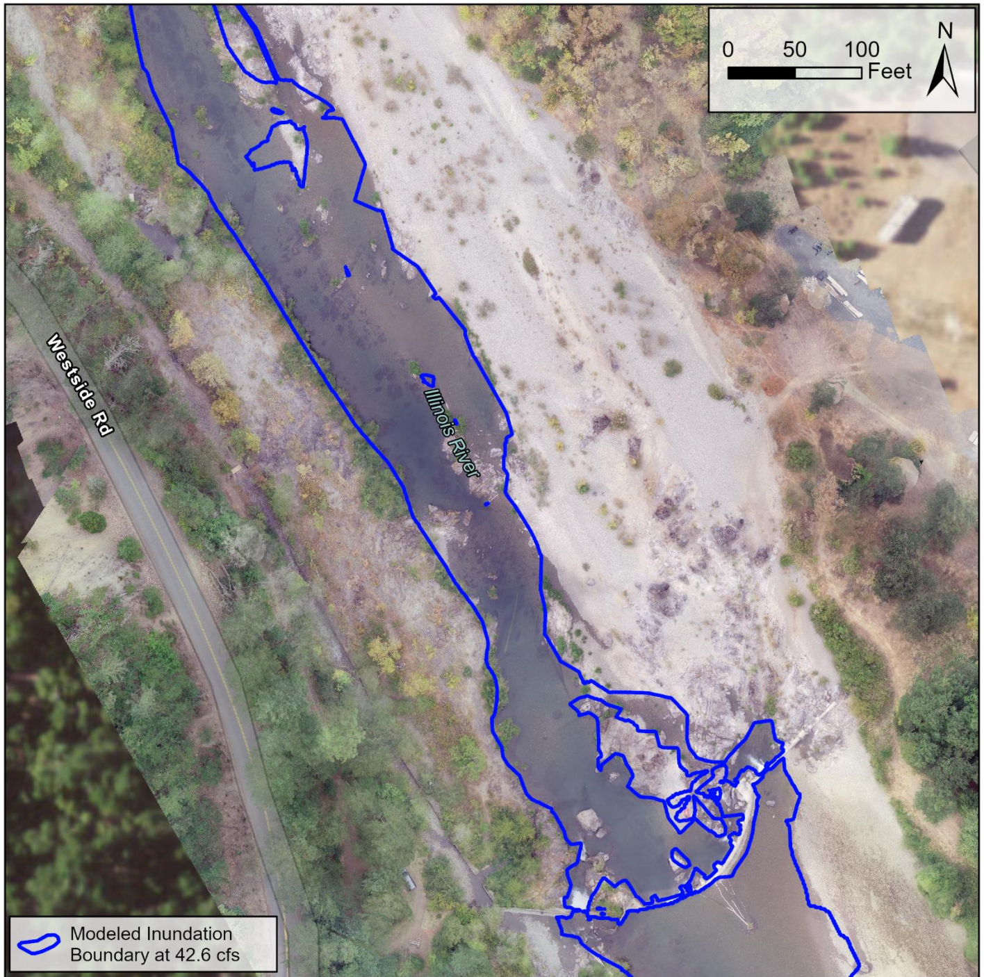
Figure 2-6. Hydraulic model validation checking the calculated inundated extents during the site survey against the observed edge of water.
